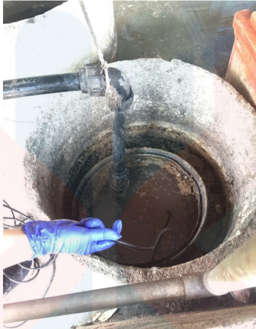
Figure A-1: In-situ analysis of the wastewater using YSI Multiparameter.
