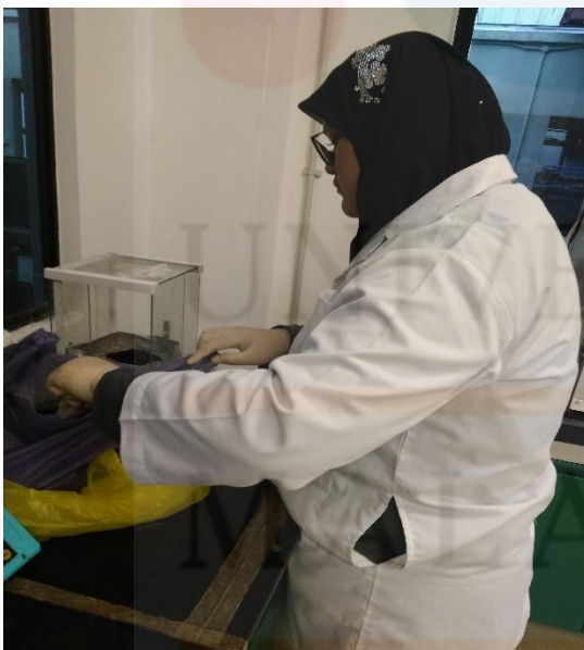
Figure B.3: Weighing the sand by using electrical weight balance
