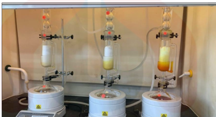
Figure 3.4 Soxhlet Extraction set up in a fume hood showing the extraction of plant rhizome samples.
