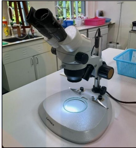
Figure 3.3: Dissecting microscope brand RaxVision used to observe microplastics on firefly
