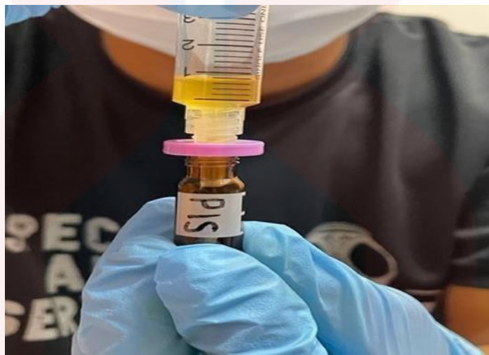
Figure 3.7: The process of filtering the sample to be inserted into the GCMS vial.
