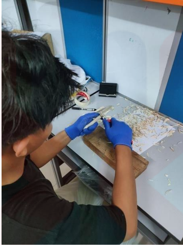
The process of slicing tree wood into smaller sizes for the steam distillation process.
