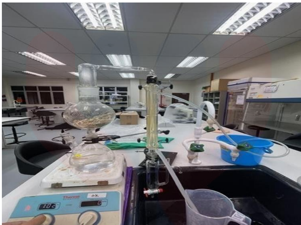
Figure 3.6: The process of extracted Agarwood oil using steam distillation process.
