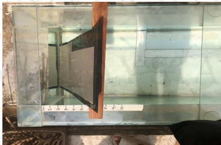
Figure 3.3: Gauge paddle use to generate wave height (above view)
