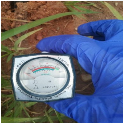
3. The pH and moisture content were measured
