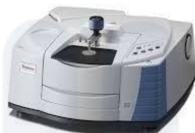
Figure 3: Shows Fourier-transform infrared spectrometer (FTIR) apparatus to identify polymer type consist in sample
