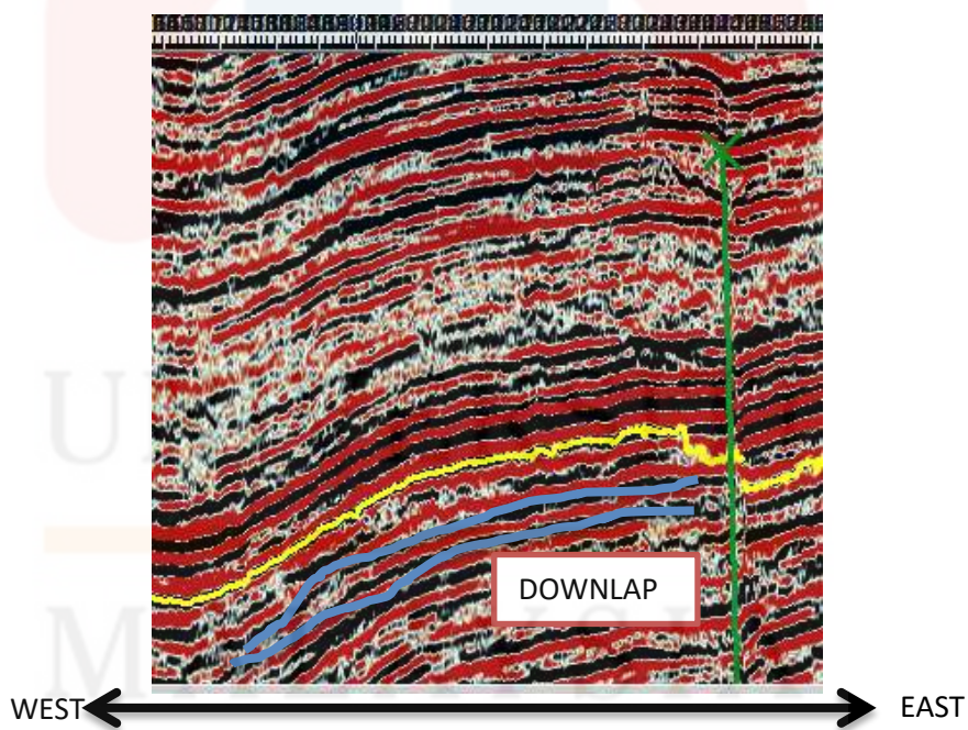
Figure 5.25: SB 2 Boundary at Inline 803
