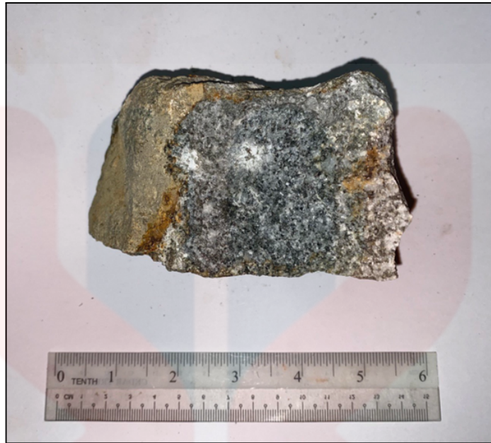
Figure 4. 6: The hand specimen of Granite, observed at station sampling day 1.
