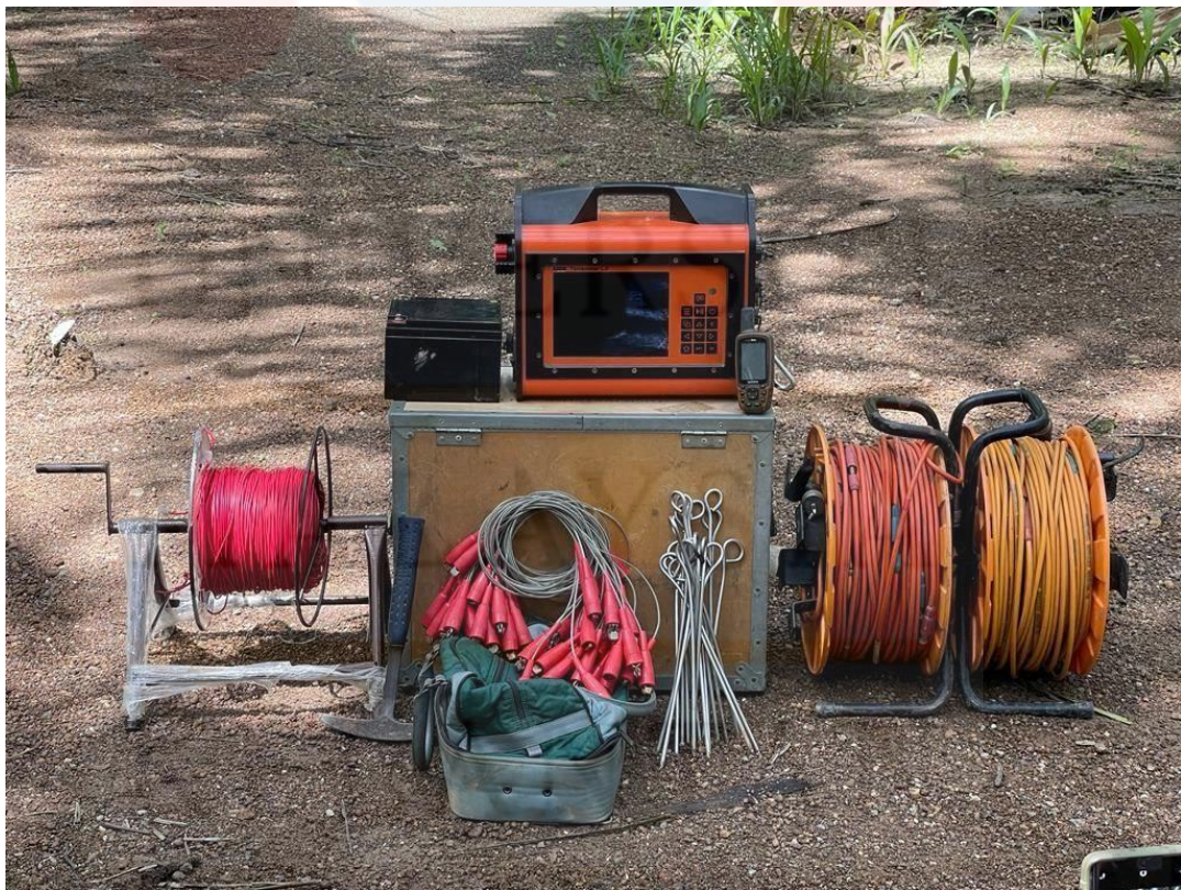
Figure 3.1: Tools & Equipment use for ERI Survey
