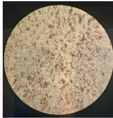
Figure 4.53: Thin section of Siltstone in 10x Cross Polarized PPL
