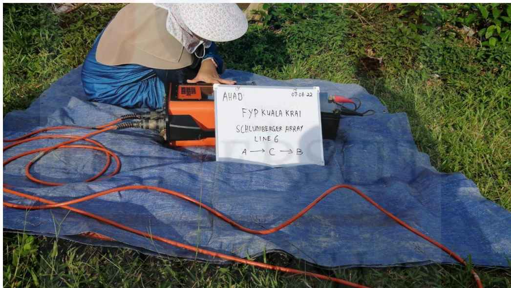
Figure 5.11: Shows the configuration setup for line survey 6
