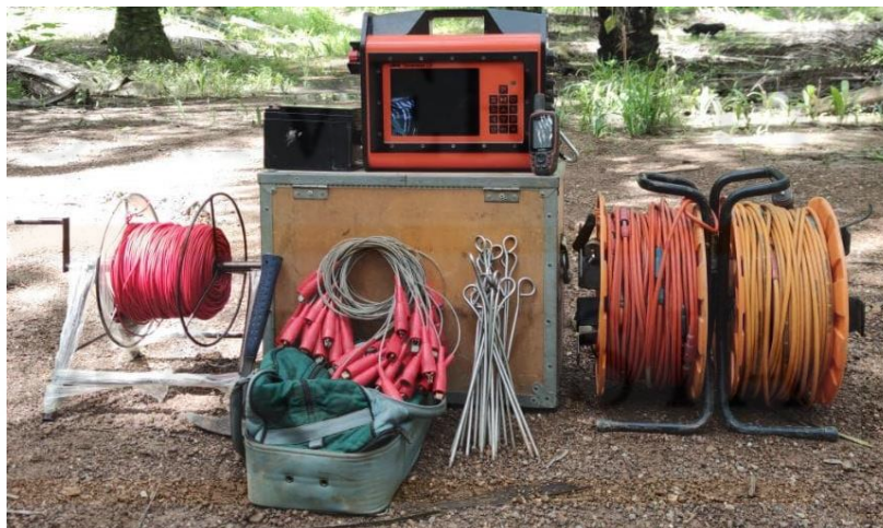
Figure 5.1: Equipment for electrical resistivity investigation.
