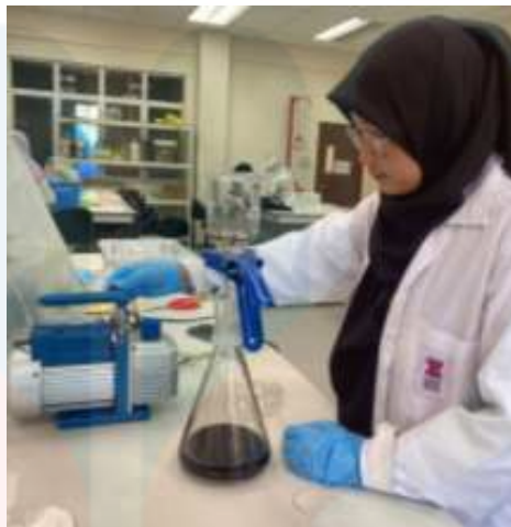
Figure 8: The filtration process to isolate the microplastics from the digested samples
