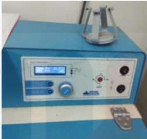
Figure 6: 25°C of temperature was set on the shaker to be shaken for 120 hours.
