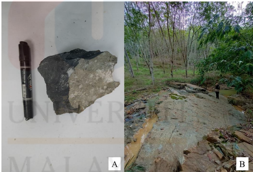
Figure 4.13: (A) Hand specimen of phyllite and (B) The phyllite outcrop in the study area.
