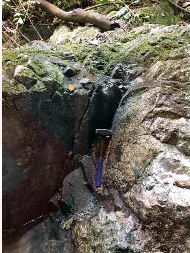
Figure 4.31 The formation of hornfels through sharp contact metamorphism
