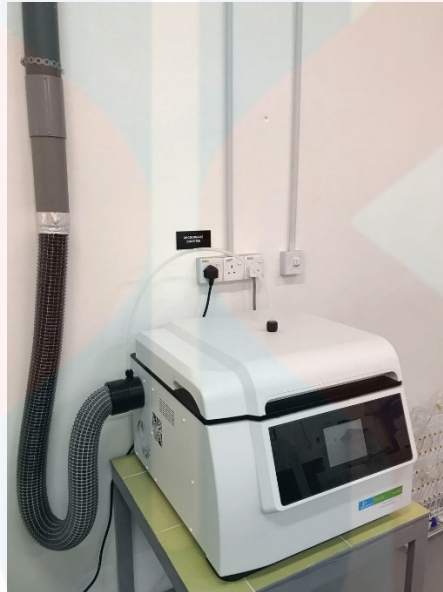
Figure 3.4 Microwave digester use to break down samples for elemental analysis.
