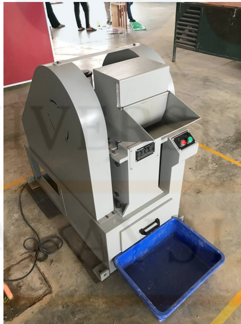
Figure 3.2 Jaw crusher use to crush granite rock into smaller size rocks.
