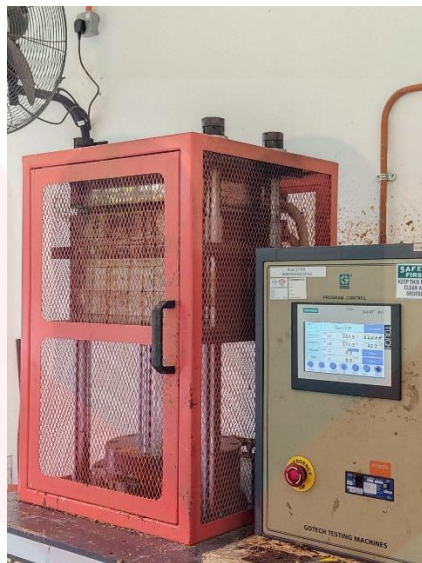
Figure 3: Using hydraulic press at temperature 180°C within 10 minutes.
