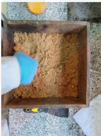
Figure 1: Particle bonded with citric acid into a particleboard measure size.
