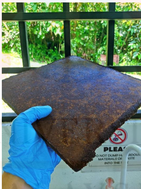
Figure 4: Particleboard made from bonded with oil bamboo particle and resin citric acid.
