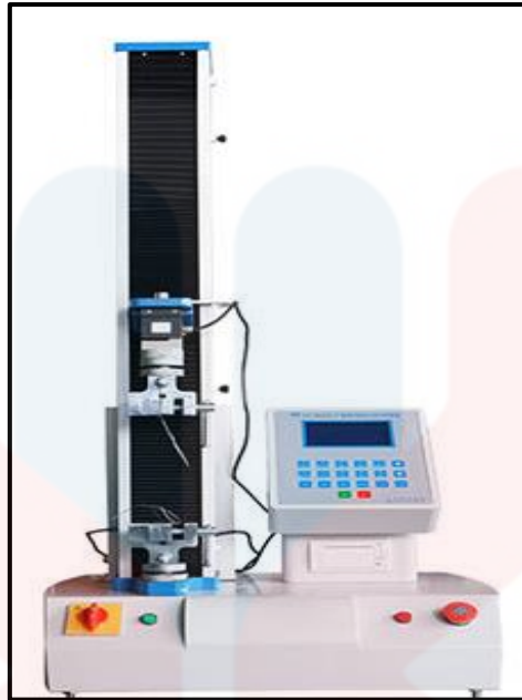
Figure 3.5: The tensile testing machine used to measure the tensile strength of the hand sheet.
