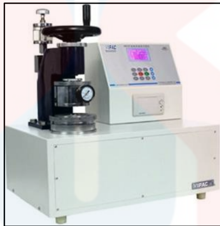
Figure 3.7: The bursting tester machine used to measure bursting strength of hand sheet.
