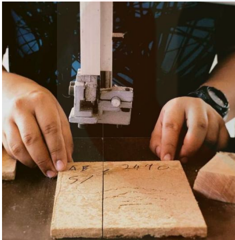
Figure A 1 : Cutting wood based composite using a table saw.
