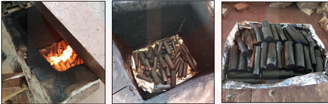
Figure 3.6 : Process of pyrolysis or carbonization of bamboo charcoal
