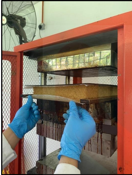
Figure A.9: The particles were put into a hot press machine.
