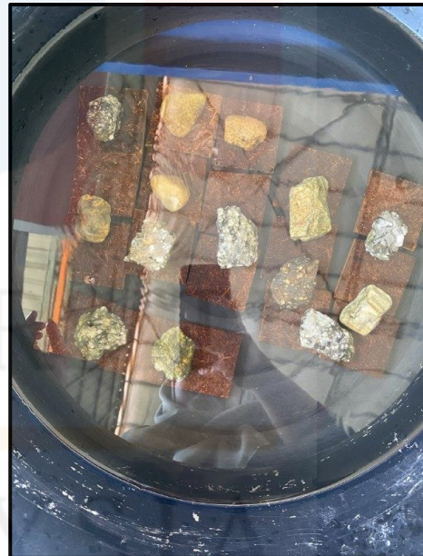
Figure A.12: Thickness swelling and water absorption process.
