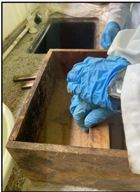
Figure A.7: Mat forming process.
