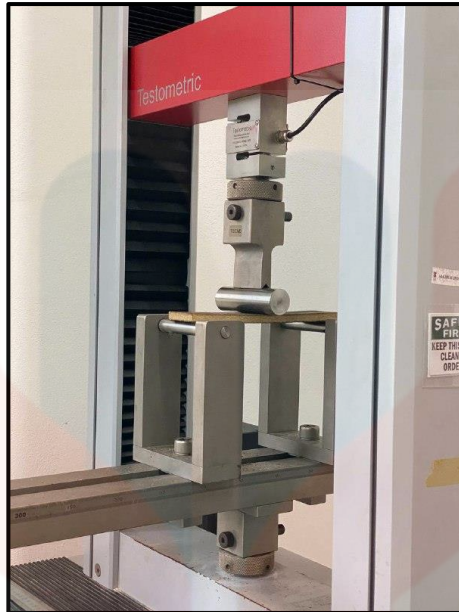
Figure A.13: Process of bending test.
