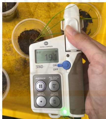
Figure 3.1 Checking chlorophyll content using Chlorophyll SPAD meter
