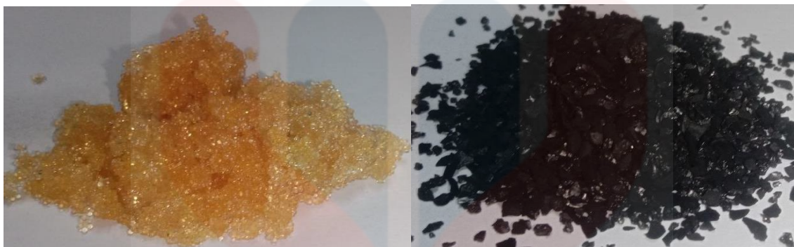
Media resin ion exchange and activated carbon
