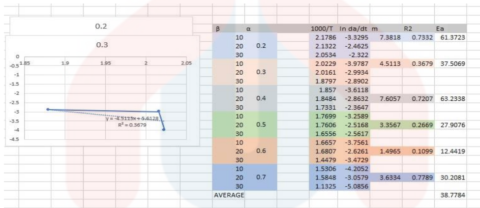
Figure 3.3 : Activation energy calculated by Friedman method for conversion 0.2-0.7
