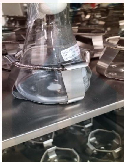
Figure 3.2: The inoculum in medium broth was incubated at 30°C in Orioner Incubator Shaker (Vis180).
