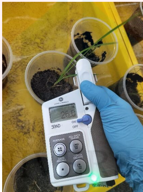
Figure 3.10: The chlorophyll content of plant leaves was measured by using Chlorophyll SPAD Meter after 14 DAS.
