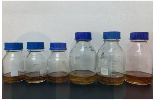
Figure 4.4 (b) : Green kenaf ribbon after degumming (24 hour)
