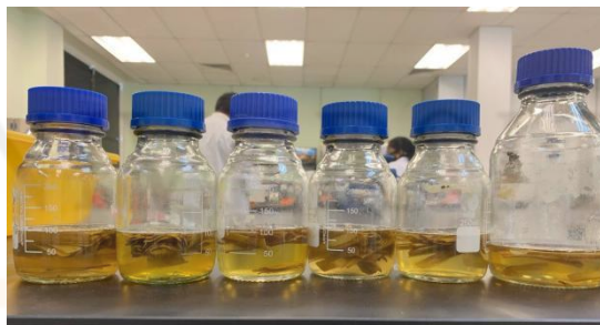
Figure 4.6 (a) : Green kenaf ribbon before degumming (72 hour)
