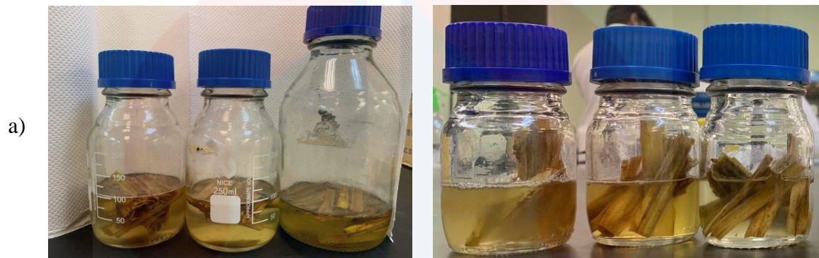
Figure 4.3 (a) : Green kenaf ribbon before degumming (0 hour)
