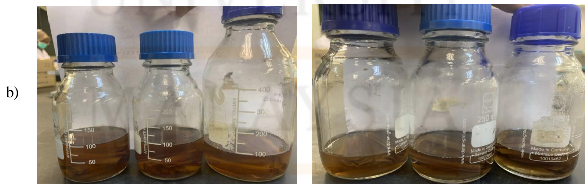
Figure 4.3 (b) : Green kenaf ribbon after degumming (72 hour)
