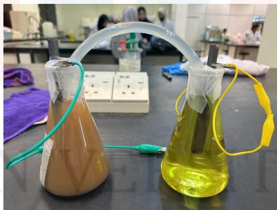
Figure A.2: Dual-chamber microbial fuel cell (DMFC) setup.
