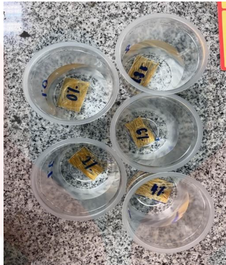
Figure 3.2: Samples of bio composites during water absorption test.
