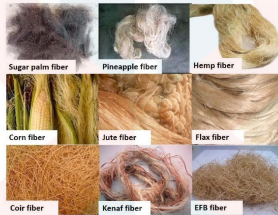
Figure 2.3: The types of reinforcing natural fibres. (Nurazzi et al.,2021)
