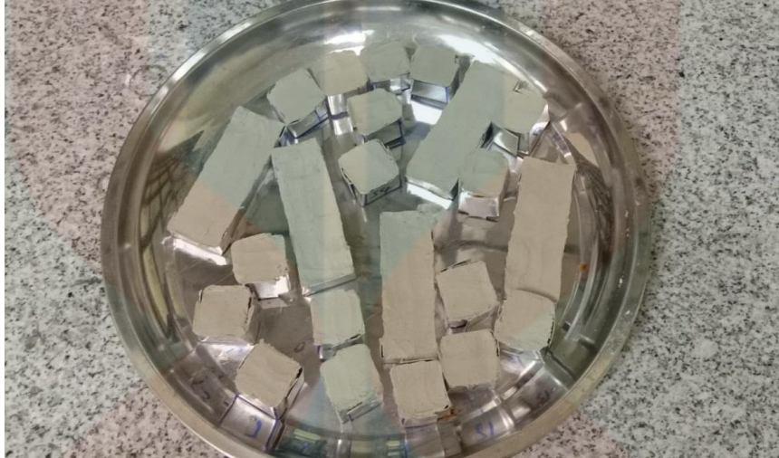
Figure A1: The ceramic bricks dried in mould before firing for 2 days.
