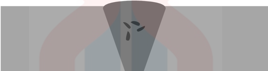
Figure 2.8: Illustration of slag inclusion
