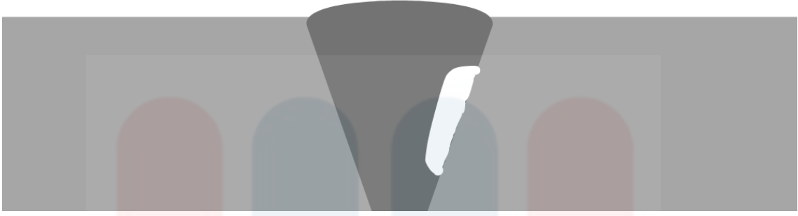
Figure 2.11: Illustration of the lack of fusion
