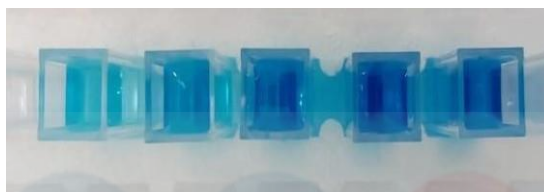
Figure 4.2: The observation of colour changes in methylene blue solution at different concentration. Cuvette arrangements from left to right are methylene blue at concentration of 2, 4, 6, 8 and 10 mg/L.
