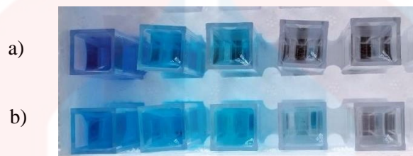
Figure 2: The observation of colour changes in methylene blue solution in different sizes. (a) 500°C/250µm/0.5g/100rpm, (b) 500°C/125µm/0.5g/100rpm
