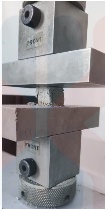
Figure A.3: Samples tested under compressive strength machine
