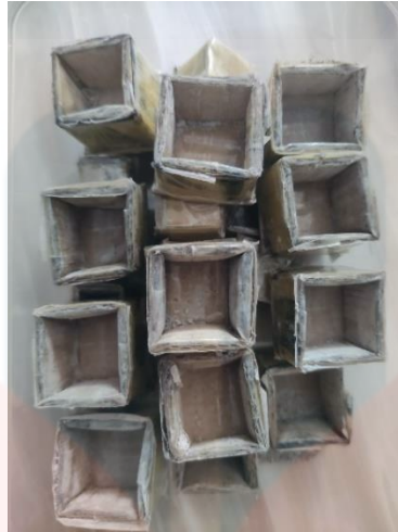
Figure A.2: Hand moulds 2×2.5×2cm dimensions
