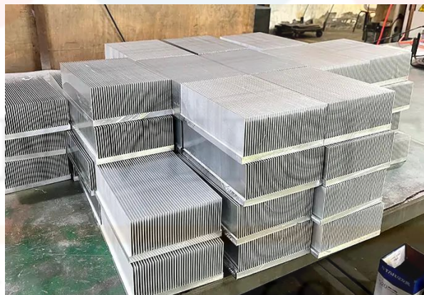
Figure 2.2: Aluminium Heat Sinks Fins ( Heat Sink Manufacturing of Xuiron, 2023 )
