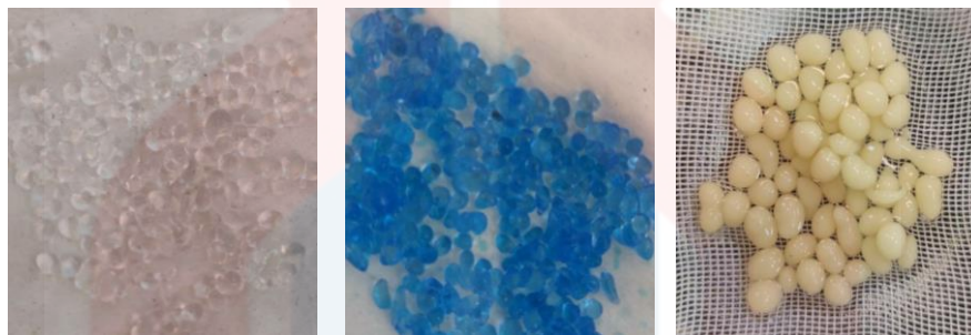
Figure B.11: The prepared calcium alginate beads: (a) Blank calcium alginate beads, (b) calcium alginate beads after treated with methylene blue solution, (c) The successfully prepared CAKB, CABC and CABB beads.
