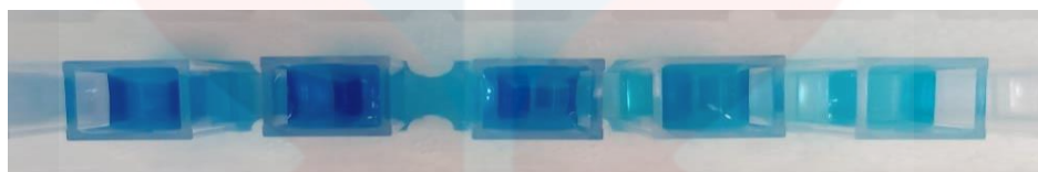
Figure 4.2: Cuvette arrangements from left to right are methylene blue at concentration of 10, 8, 6, 4 and 2 mg/L.
