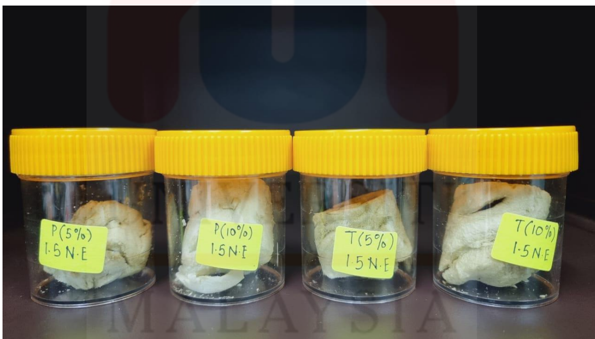
Figure A4: Starch aerogel samples incorporated with 3% Neem leaf extract.
