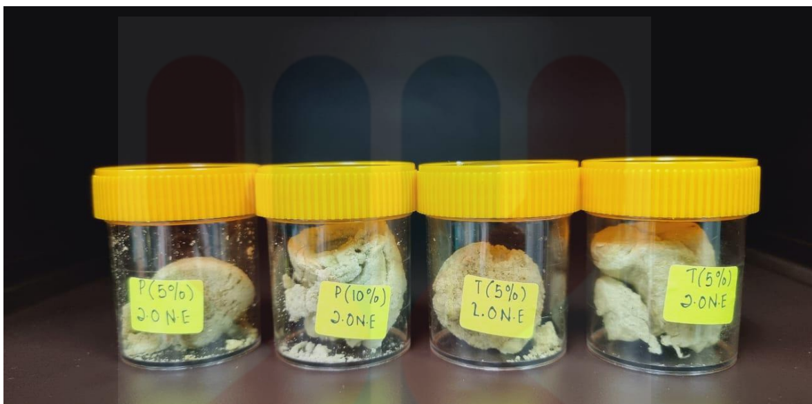
Figure A5: Starch aerogel samples incorporated with 4% Neem leaf extract.
