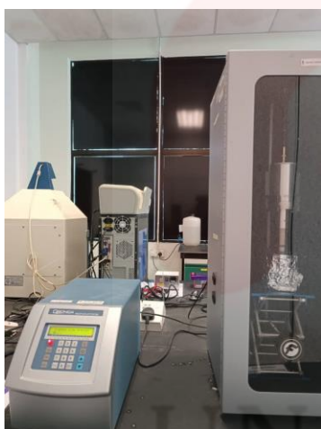
Figure C.3: Sonicator for the effective dispersion of the samples
