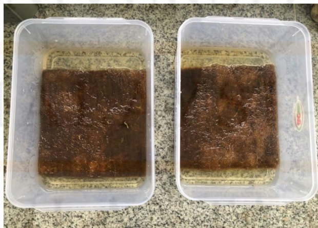
Figure 3.1: KFM immerse in sodium hydroxide (NaOH).
