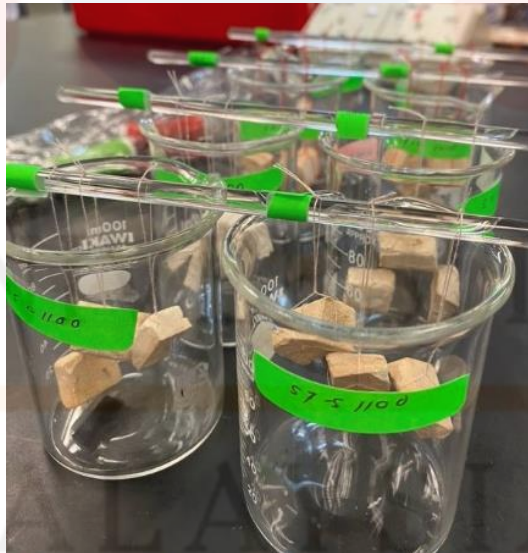
Figure 3.12: Ceramic brick sample suspended on a glass rod into a beaker.
