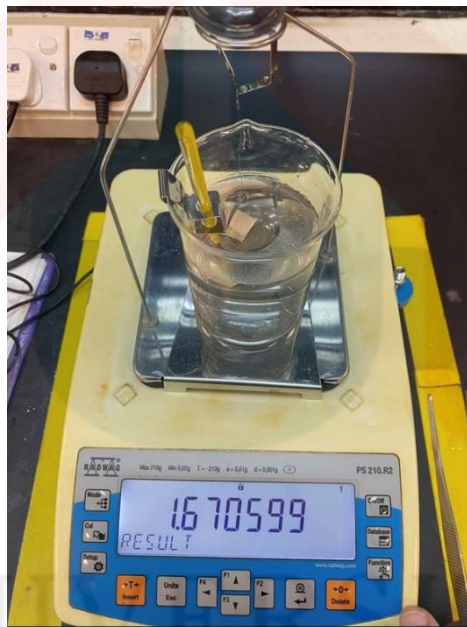
Figure 3.15: The density of sample was measured using density determination set.
