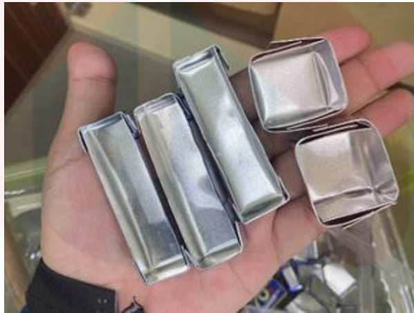
Figure 3.6: Two size of handcrafted mold (60mm x 15mm x 1mm) and (25mm x 25mm x 20mm).
