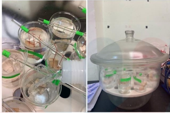
Figure 3.13: Distilled water has been poured into the beaker and let the samples submerged completely.
