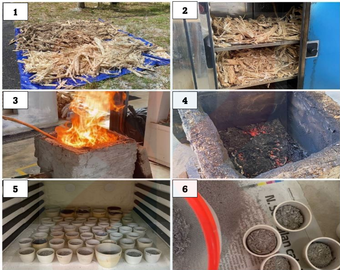
Figure 3.2: Process involved in investigating sugarcane bagasse ash formation.
