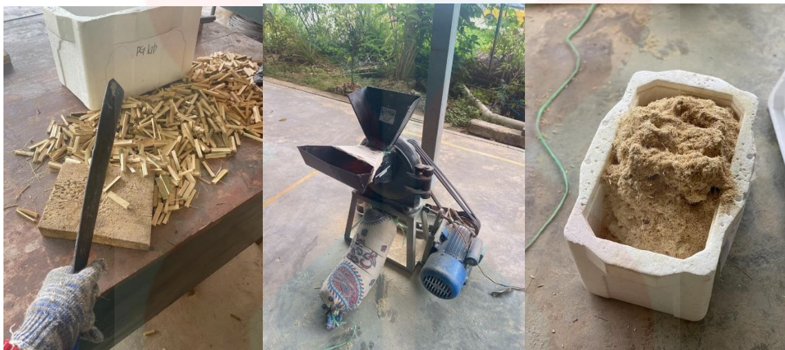
Figure B.1 : Preparation carbon black from bamboo
