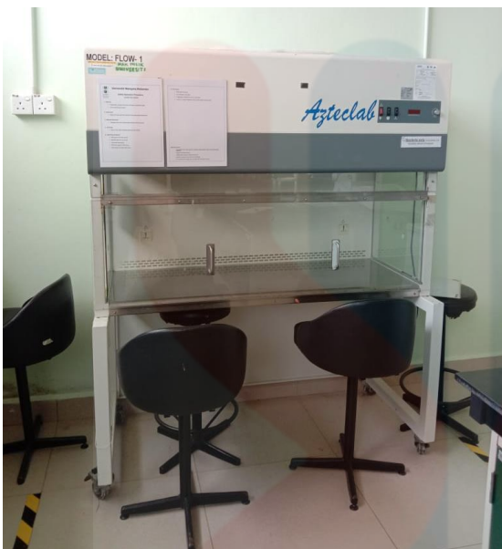
The laminar flow used in preparation of media and serial dilution in aseptically technique
