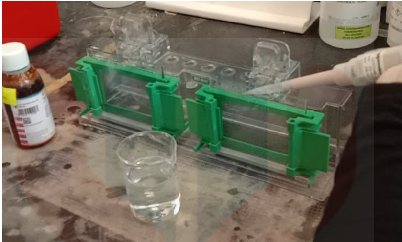
Figure B.9: Process of pipetting the gel into the casting plate for SDS-PAGE
