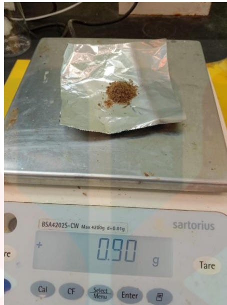
Figure B.3: Sample was weighed using an electronic weighing scale
