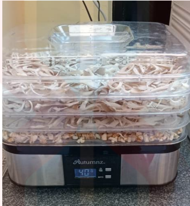
Figure A.1: Drying of sample using dehydrator machine at 40°C in 24 hour
