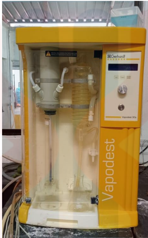
Figure A.5: Gerhard Analytics machine for nitrogen analysis
