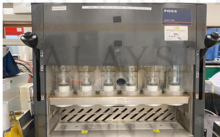
Figure A.7: FOSS analytical ST 255 Soxtec™ used to extract fat in the sample
