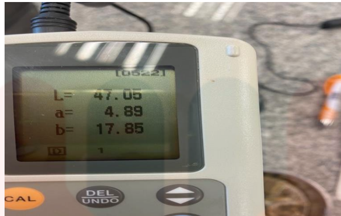
Figure A.10: Colour characteristics of the sample were tested and L, a, b scale were displayed at CR-400 Chroma Meter
