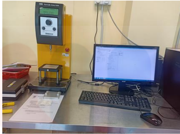
Figure A9: Brookfield CT3 Texture Analyser with cylinder probe used to determine the hardness of formulated egg custard
