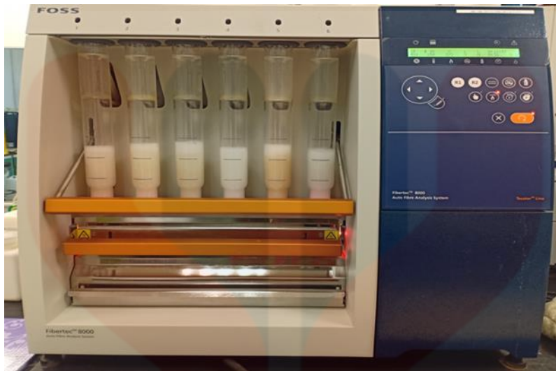
Figure A7: FOSS Fibertec™ 8000 machines used for identify crude fibre in sample.
