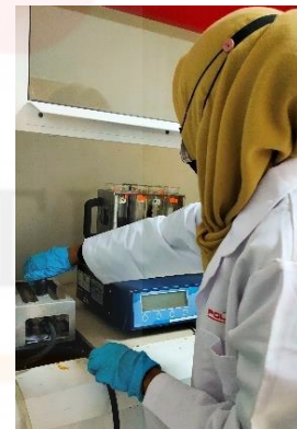
Process of digestion in CP analysis
