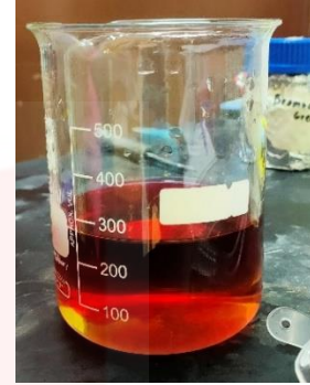
Bromocresol green and Methyl red solution as a receiver for distillation process in CP analysis
