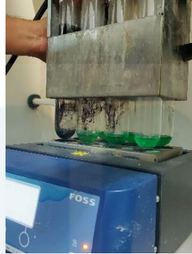
Result of digestion process in CP analysis
