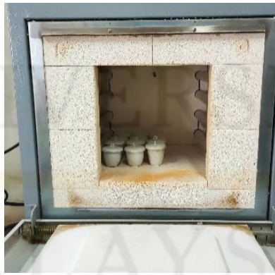
Muffle furnace for Ash analysis
