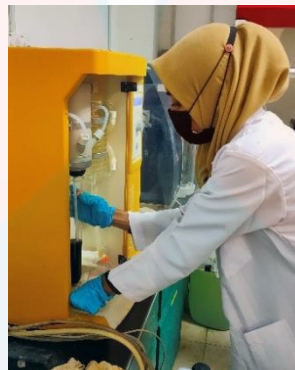
Distillation process in CP analysis
