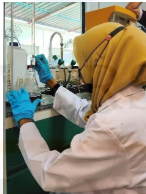
Process of titration to know the amount of N in sample
