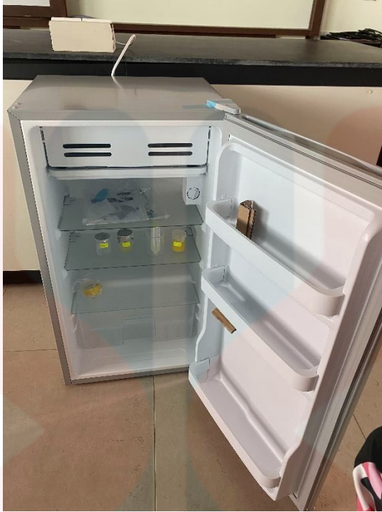
Figure 3.9: Storing of TCFY solution in chiller at 4°C
