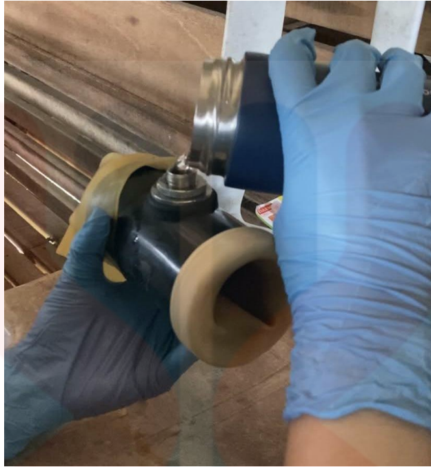
Figure 3.11: Adding of warm sterile water into space between the sleeve and cylinder of AV
