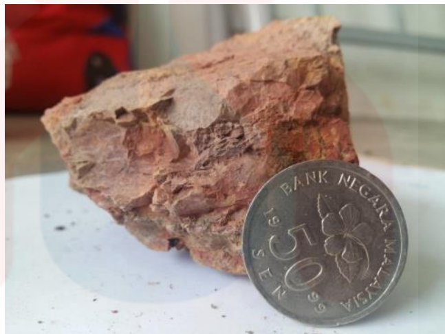
Figure 4.13: Hand specimen of shale from Shahman (2017).
