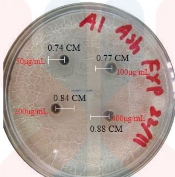
Figure 2 Zone of Inhibition Aspergillus versicolor on Sabouraud Dextrose Agar (SDA) treated with Graphene Oxide after 24 hours
