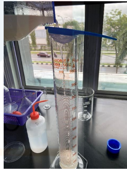
Appendix A.8: Filtration of digestion fluid
