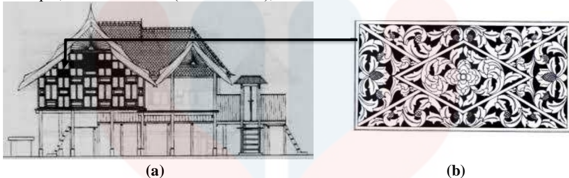
Figure 1: The layout of carved components at wall facade of rumah ibu at Mohamad Dobah’s house (a) and one of carved ventilation panels (b) found on the wall
