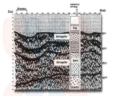
Figure 5.4: Interpretation of seismic section and lithology in Bachok, Kelantan
