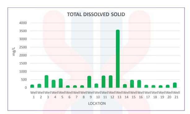
Figure 5.13: TDS measured the in the sampled wells
